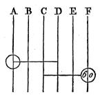
which means that an adjustment is to be made by fixing A on its axis, making a right angle with D, and that F must also make with C an angle of sixty degrees. In speaking of these angles, it should always be observed that they refer to the angles made by the parts on one of the planes of projection.
